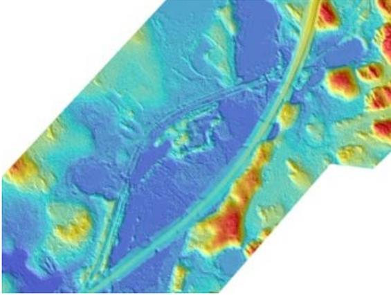
*[LiDAR data used to identify ice-rich permafrost terrain.](#)*
