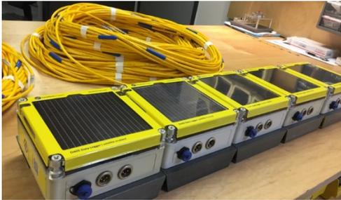
[\*Data loggers and cables used to monitor ground temperature changes beneath critical infrastructure constructed in permafrost environments.\*](#)
