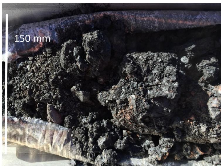
Figure 6 H9 carbonaceous mudstone core
