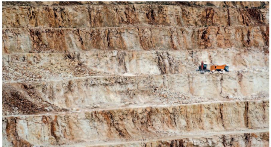
A geotechnical model should be developed based on a thorough understanding of the geology, structure and, where relevant, alteration and weathering states of the deposit and how these impact the engineering properties
