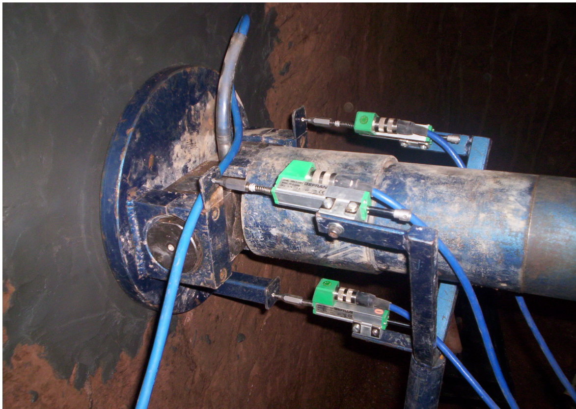
Fig. 5. Plate load test, Line B, 2006.
