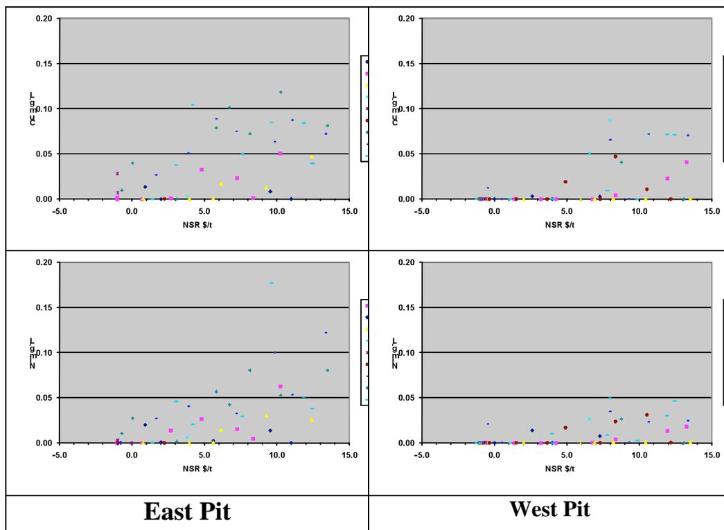
Figure 5: Release of nickel and copper from the NAG test
