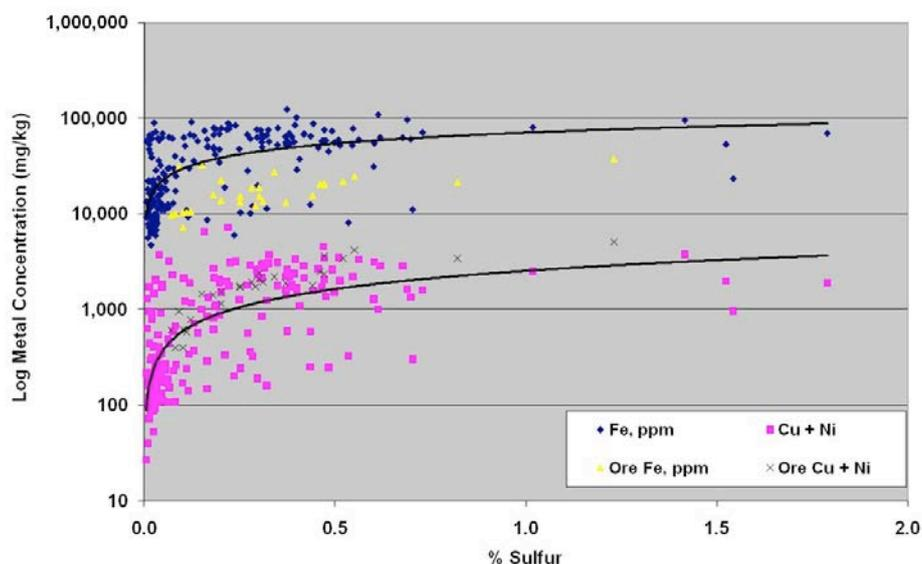
Figure 3: Relationship between copper, nickel, iron and sulfur
