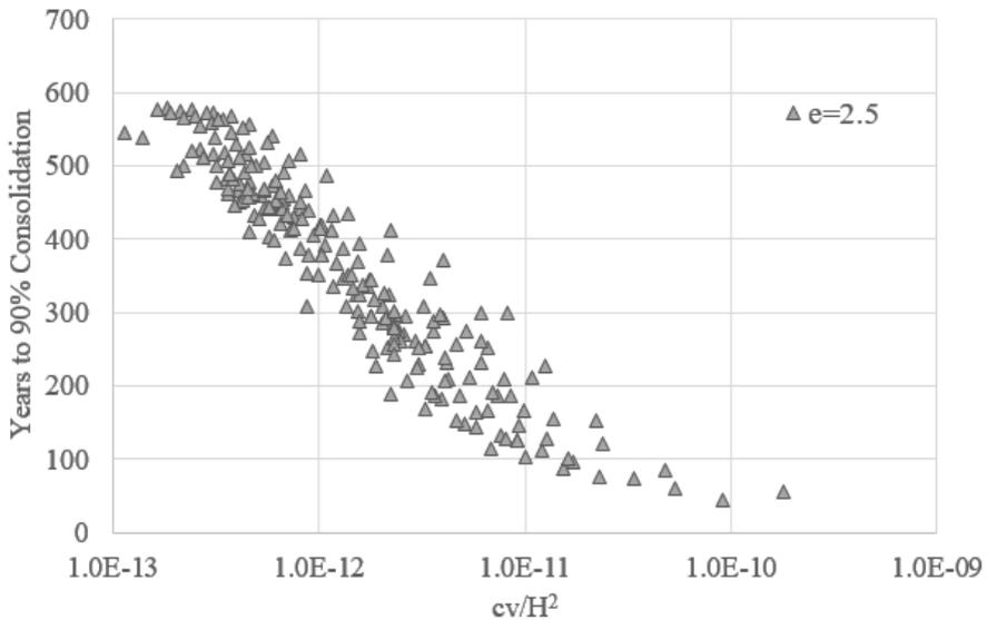
Figure 7. Consolidation time versus  $c_v/H^2$  <sup>1</sup>
