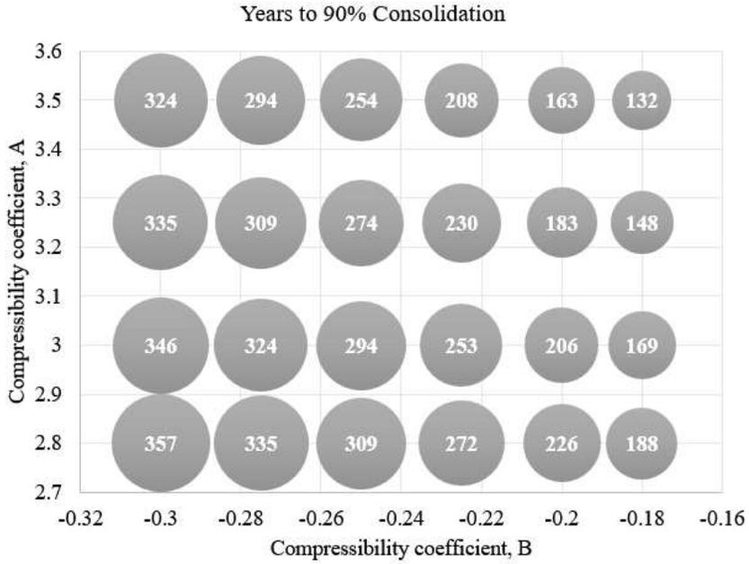
Figure 4. Effects of compressibility parameters on time to reach 90% consolidation
