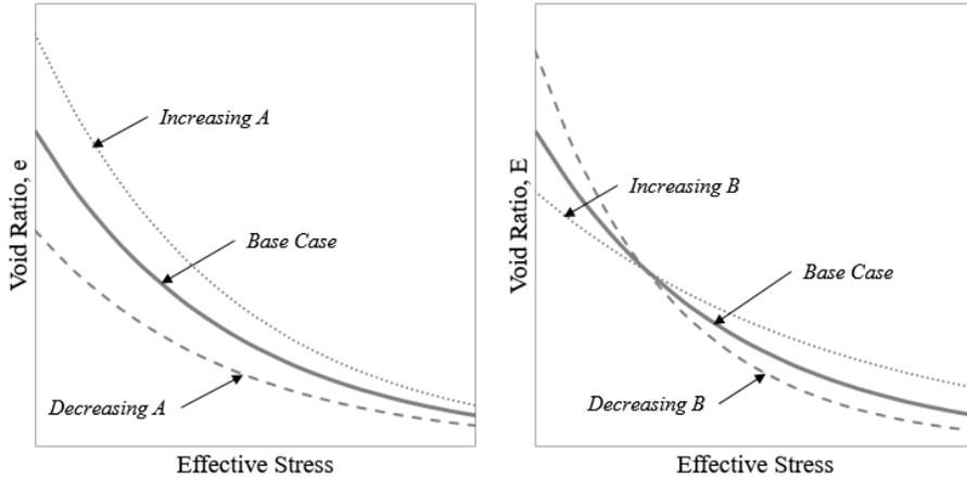
Figure 1. Effect of A and B values on compressibility
