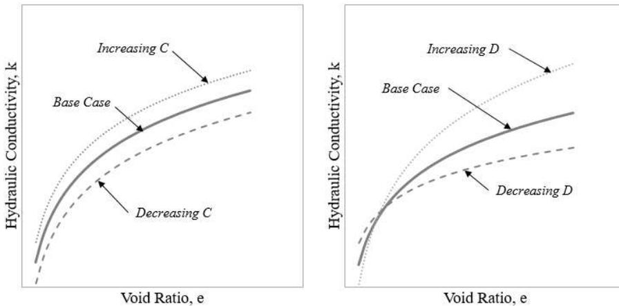
Figure 2. Effect of C and D values on hydraulic conductivity
