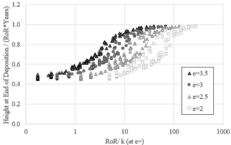
Figure 6. Dimensionless rate of rise vs dimensionless deposit height
