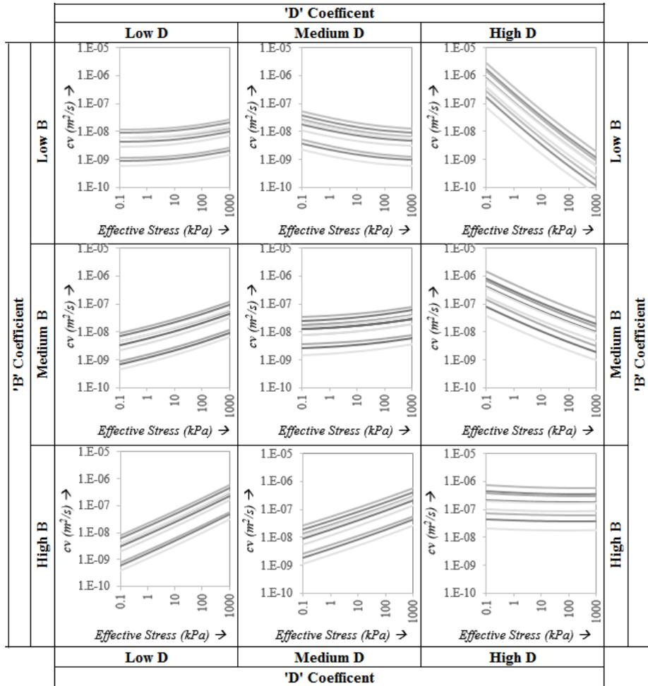
Figure 8. Coefficient of consolidation ( $c_v$ ) functions from 700 sensitivity runs
