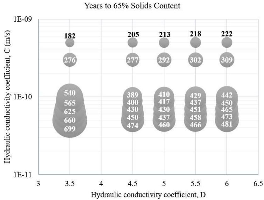
Figure 5. Effects of hydraulic conductivity parameters of time to reach 65% solids
