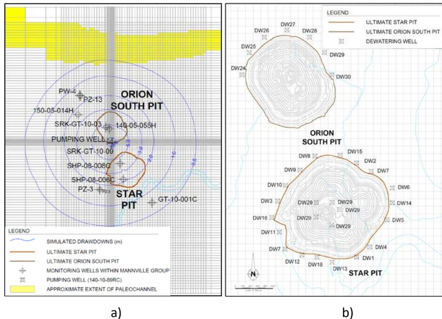
**Figure 4** (a) Drawdown at the end of pumping test and (b) location of simulated dewatering wells
