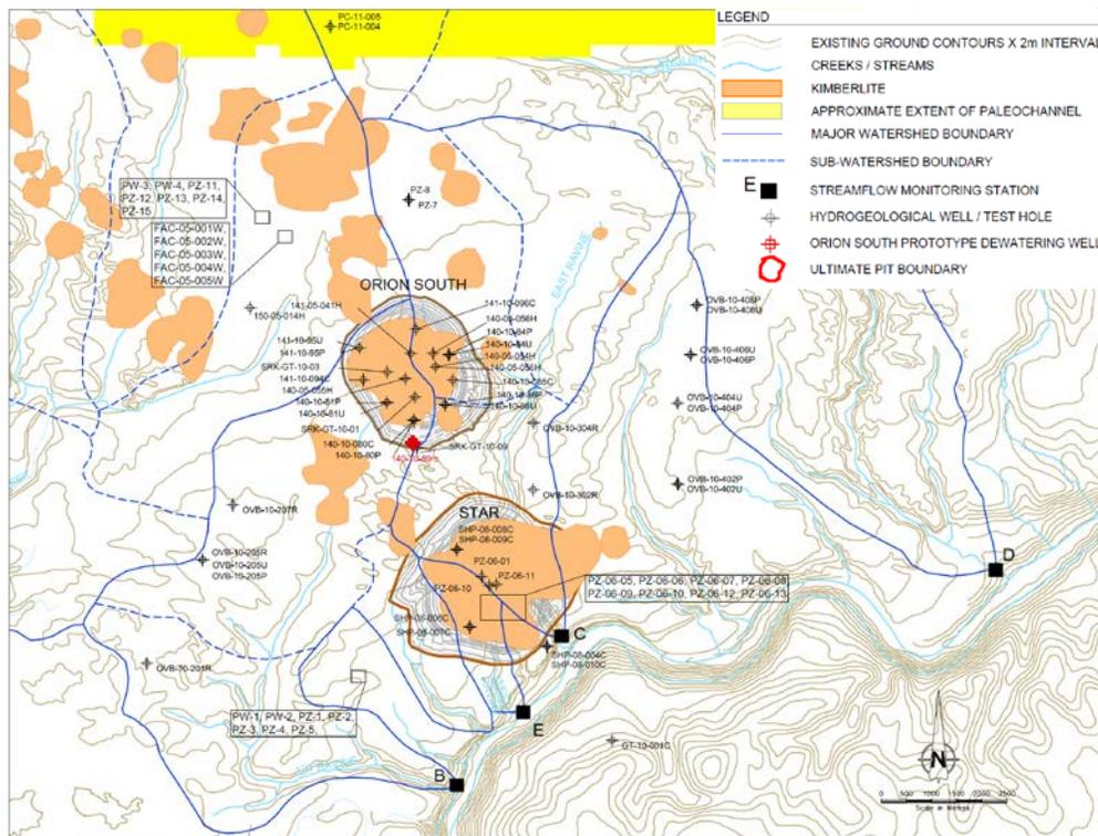
**Figure 1** Location of proposed open pits and completed hydrogeological wells
