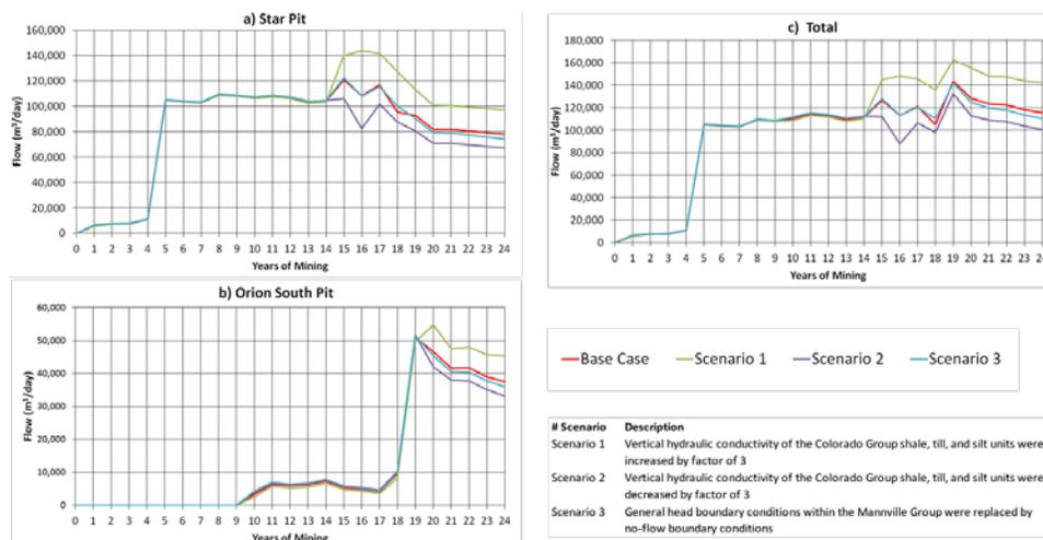
**Figure 6** Results of sensitivity analysis of hydrogeological parameters on predicted dewatering
