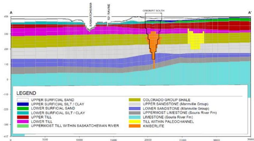
Figure 2 Hydrogeological units incorporated into numerical groundwater model
