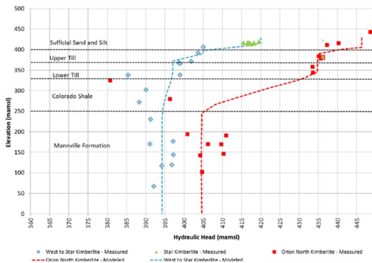
Figure 3 Comparison of measured and modeled water levels vs. elevation for two sites
