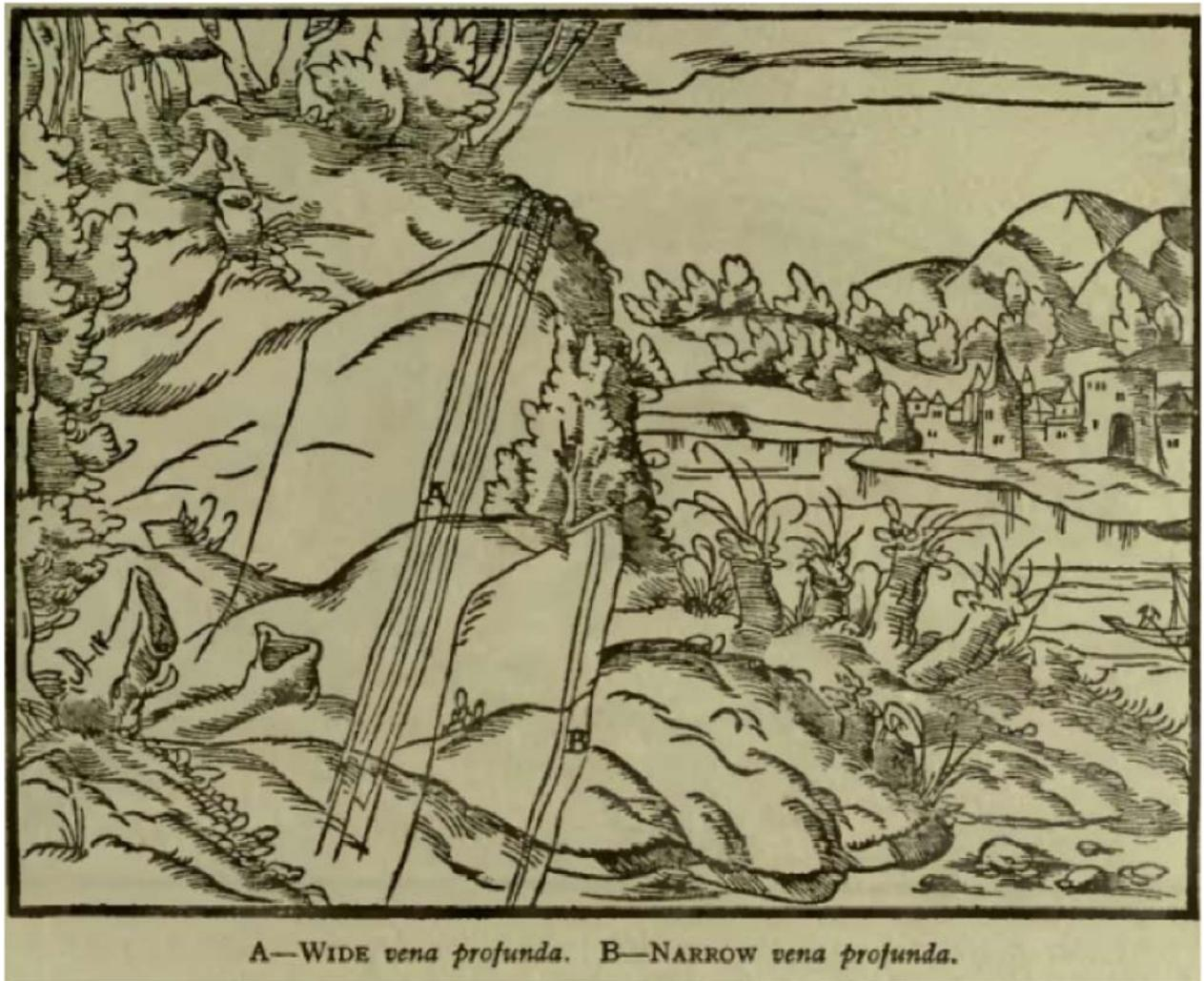
Figure 1. Wide and narrow veins as illustrated in De Re Metallica circa 1556.
