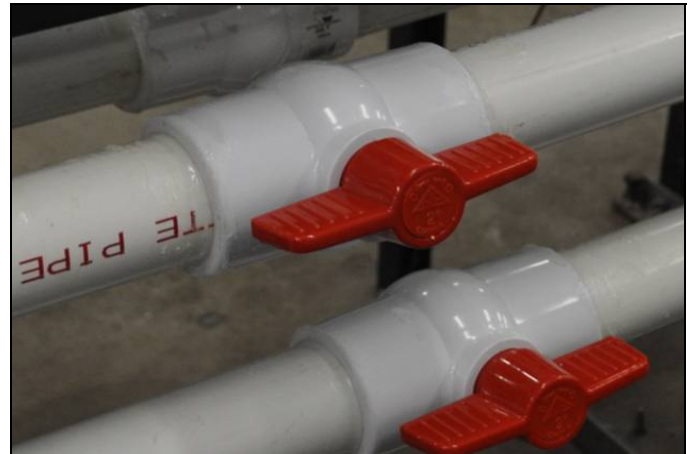
Figure 4. Valves Are Used to Simulate Ventilation Controls and Mine Airway Damage.
