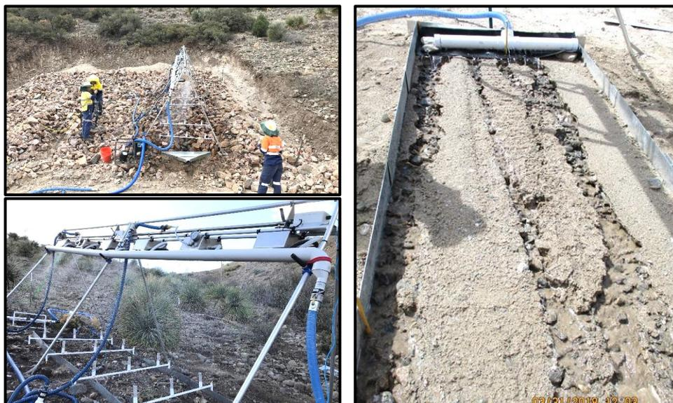
**Figure 3** Rainfall simulations and overland flows being applied to test surfaces.
