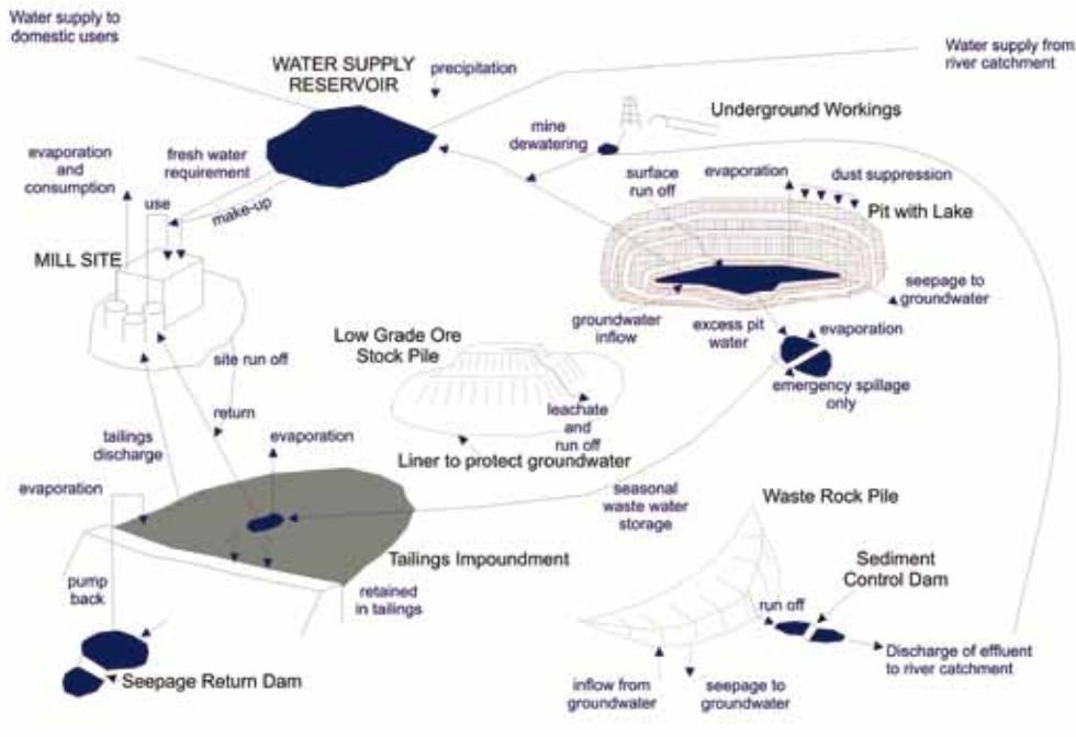
**Conceptual relationships in a mine water balance (adapted from Smith and Mudder, 1991)**
