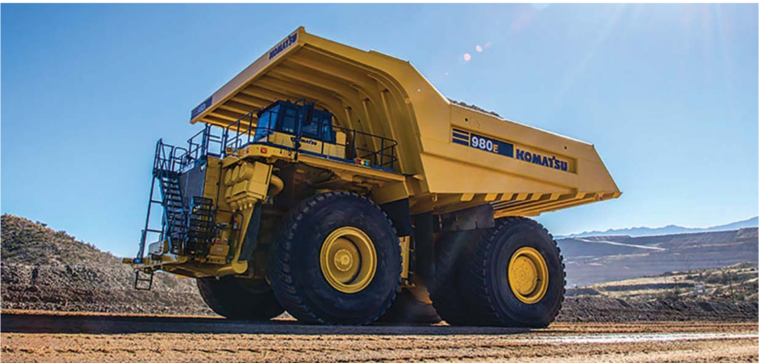
Bigger is still better, but only in certain circumstances. Komatsu's 980E-4, above, offers a 400-short-ton payload.
