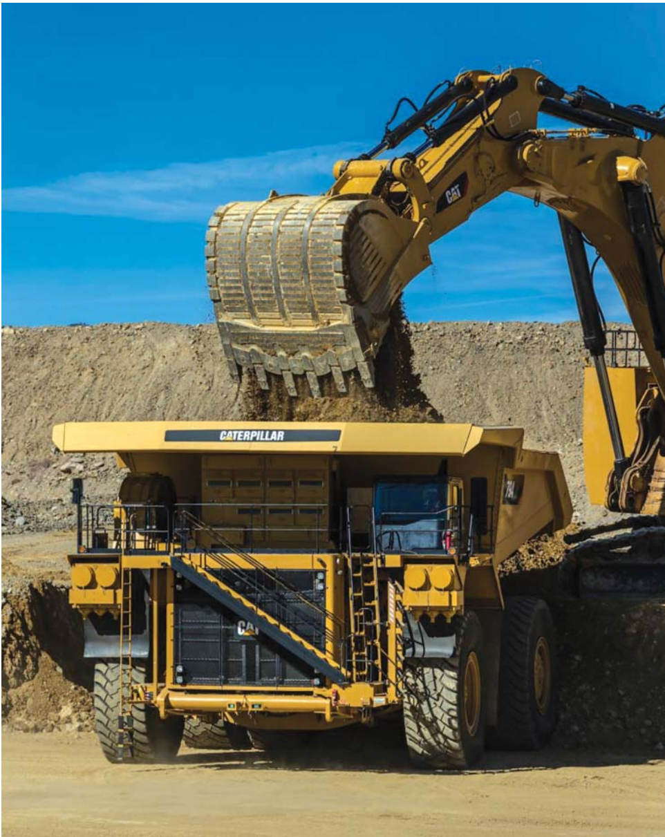
Ramp slope, road conditions, maintenance costs, and fleet management challenges should all be considered when planning to deploy an ultra-class truck, two mining engineering professors say. Above, a Caterpillar 794 AC tops off.
