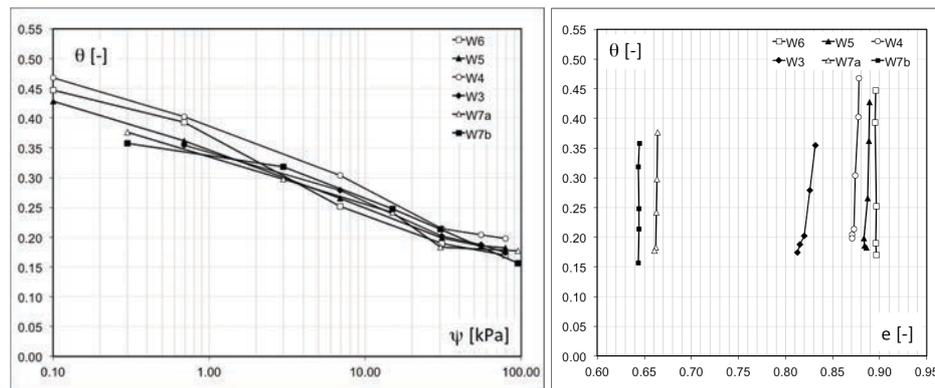
**Figure 8.** (a) Soil-water retention curve ( $\theta$ - $\psi$ ), (b)  $\theta$ - $e$  relationship.
