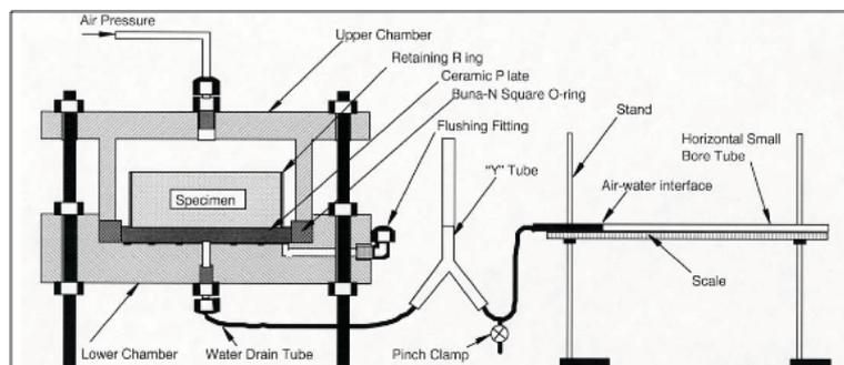
Figure 1. Schematic of Pressure Extractor ASTM D6836-02 (2008).
