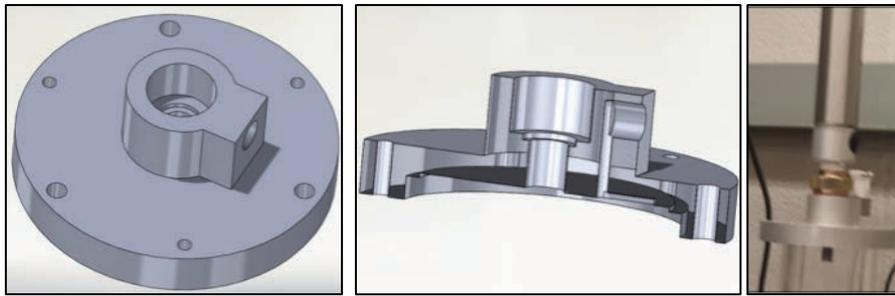
**Figure 4.** a) 3D view of the cap, b) cross section, and c) piston connected to the cap.
