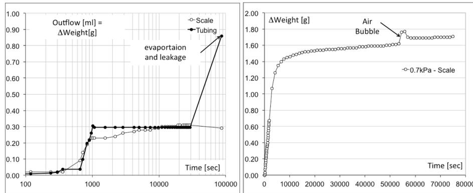
**Figure 11.** (a) Comparison of measurement systems. (b) Dynamic response of the scale due to air bubbles.
