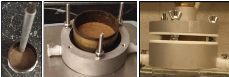
**Figure 3.** a) Compaction, b) sample mounted in the base, c) base assembled with the top disc and o-ring holders.
