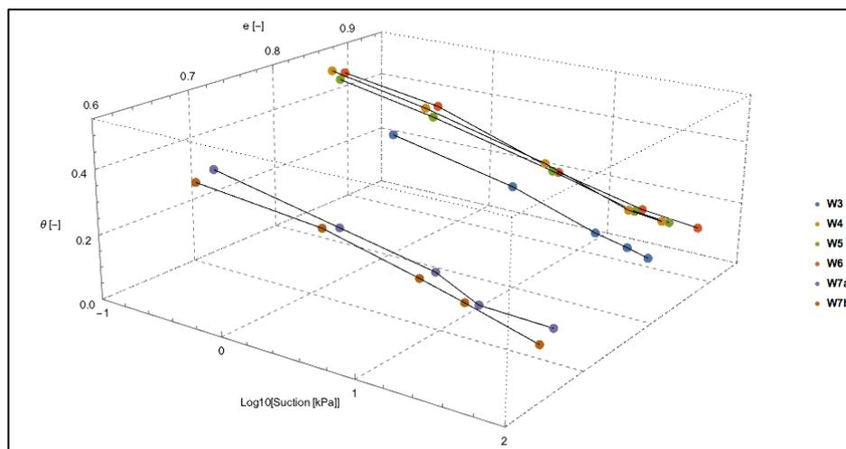
**Figure 7.** Multiple stages on wetting hydro-mechanical path.
