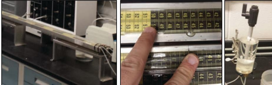
**Figure 5.** View of: outflow capillary tubes (a), readings affected by bubbles (b), and air trap connected to the flushing system(c).
