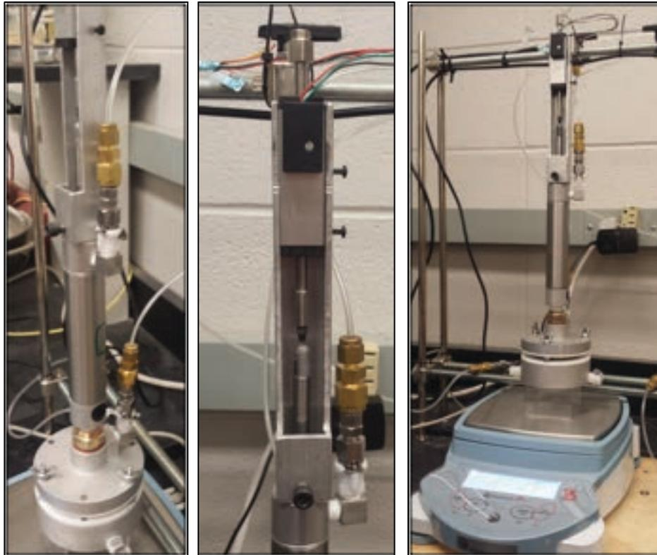
**Figure 6.** View of the piston and air connections (a); detail of the bracket and LVDT (b); and complete chamber mounted over the scale (c).
