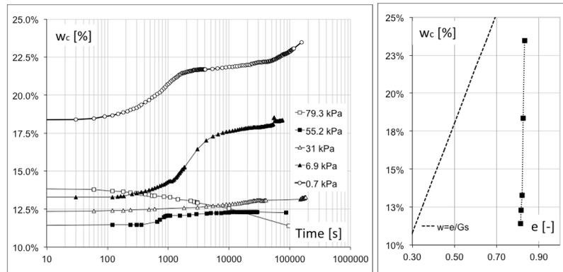
**Figure 10.** (a) Evolution of gravimetric water content with time, (b) relationship between water content and void ratio at the end of each stage.
