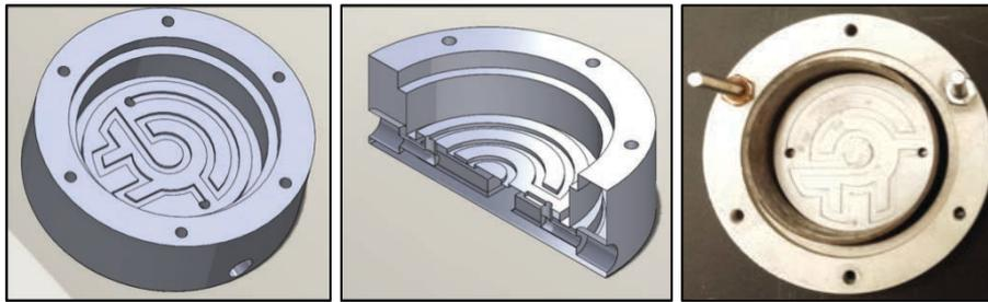
**Figure 2.** Base detail: a) 3D view of base design. b) Cross section showing grooves, inlet, and outlet connections. c) Picture of the base.
