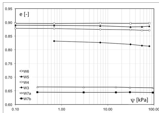
**Figure 9.** Changes in void ratio with suction ( $e$ - $\psi$ ).
