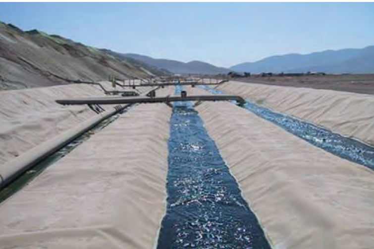
Figure 5 Typical solution collection channels and piping
