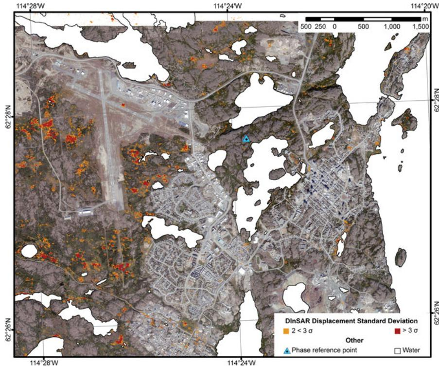
FIG. 3. DInSAR standard deviations ( $> 2 \sigma$ ) of seasonal surface displacement overlaid on 3.2 m resolution IKONOS satellite image of Yellowknife acquired August 21, 2005. Note the IKONOS image has a slightly limited northern extent. Satellite image courtesy of GeoEYE ([www.geoeye.com](http://www.geoeye.com)). © GeoEYE. Reproduced by permission of GeoEYE. Permission to reuse must be obtained from the rightsholder.
