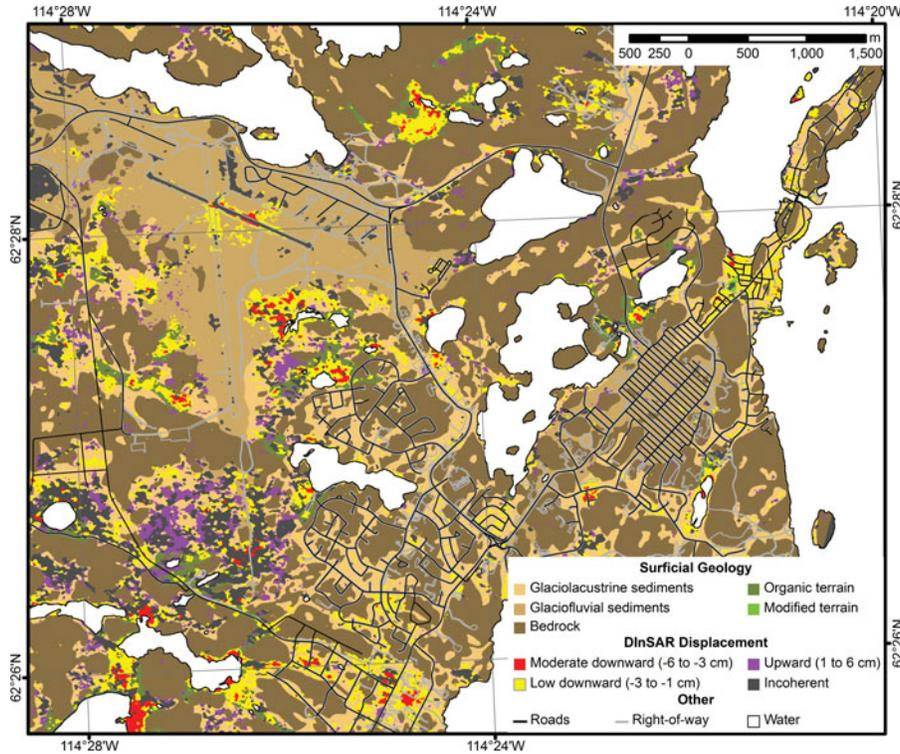
FIG. 5. Surficial geology overlain with DInSAR seasonal surface displacement. DInSAR stable areas are omitted in order to reveal the surficial geology.
